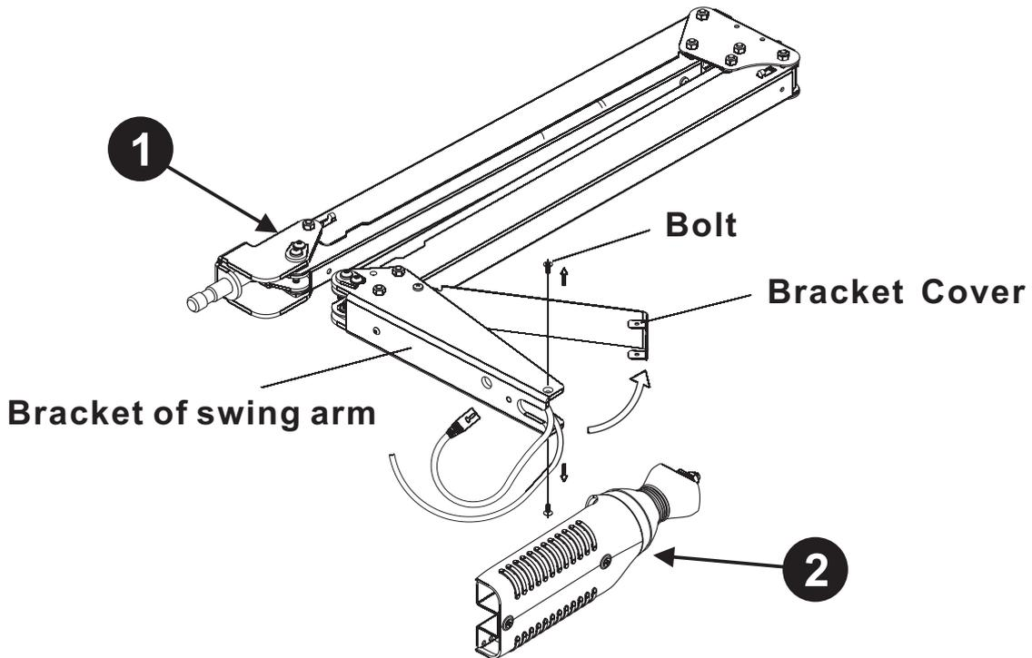
Remove the screws from the swing arm covers, and lift the bracket cover at the main arm.
