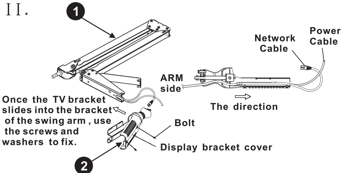
Once the TV bracket slides into the bracket of the swing arm, use the screws and washers to fix.
