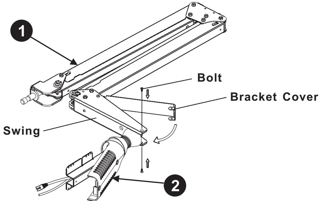
Once the electric wire is in the right position, then cover the bracket cover and use the bolt to tighten the two sides of the main swing arm.
