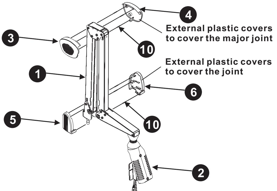
Take three pcs of pin to press and fix the external plastic covers according to the location, that shown from the drawing.
