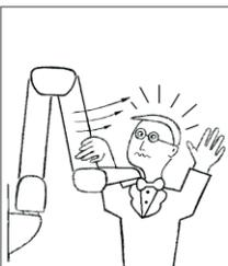
**WARNING:** This arm contains internal springs under tension. AN ARM RECOIL ACCIDENT HAZARD IS POSSIBLE. FOLLOW ALL SAFETY INSTRUCTIONS AT ALL TIMES.
