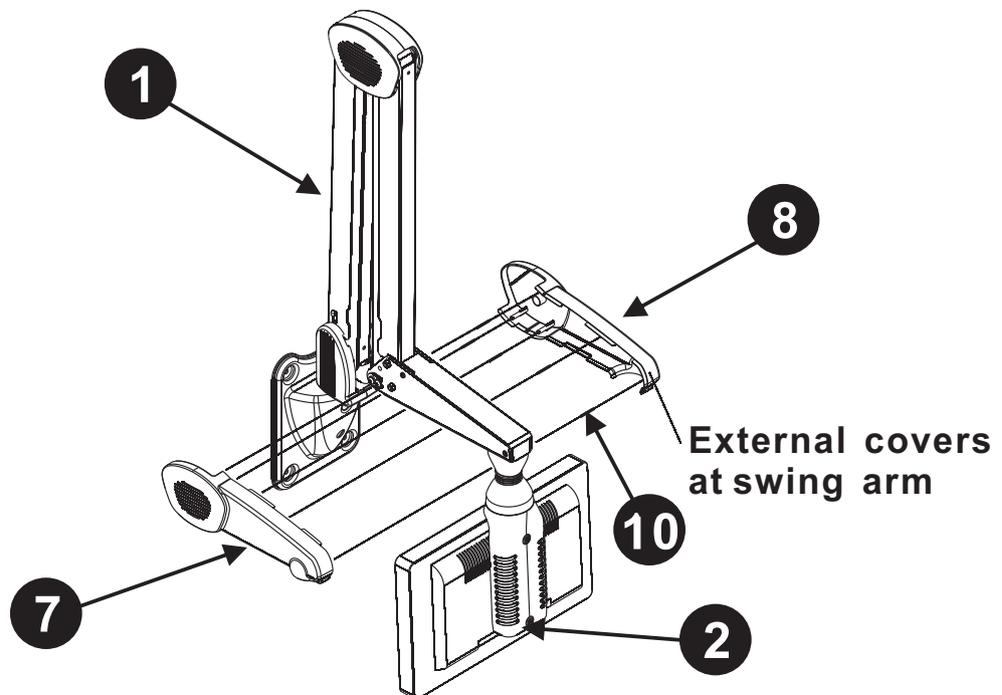
Take five pcs each of pin and swing arm external covers push, Press to the fix feature according to the location shown from the picture.
