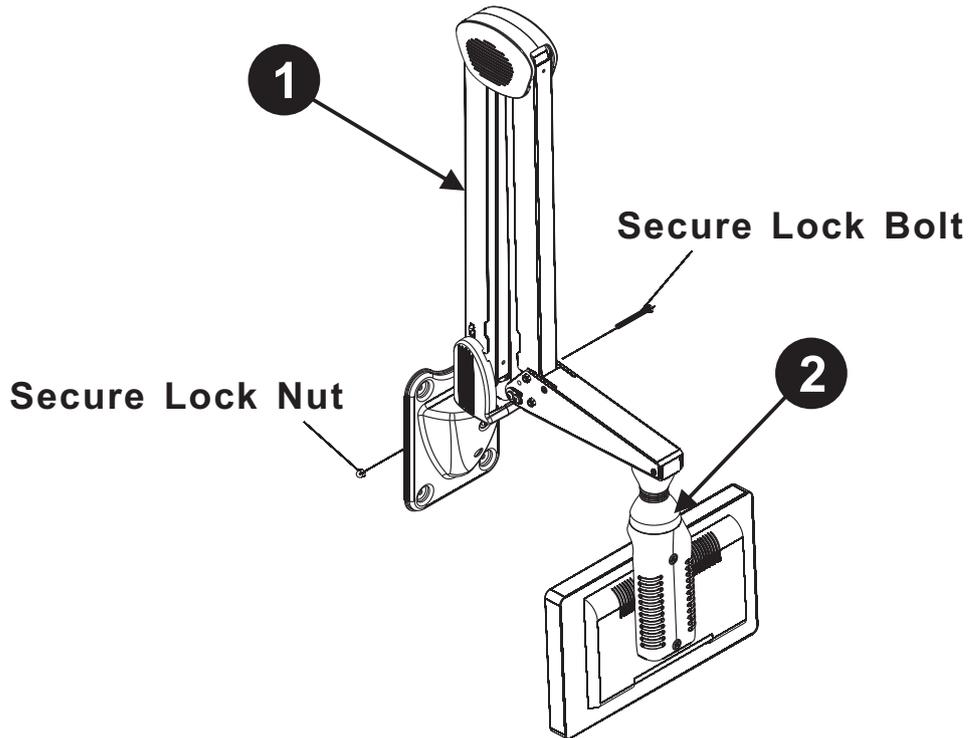
Remove the secure lock nut and bolt.
