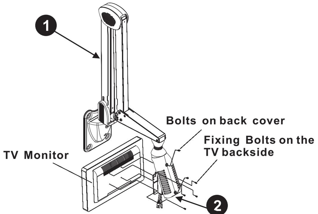
Use four Bolts to fix the TV monitor, then use two Bolts to fix the back covers. Connect the electric wire with the slot.
