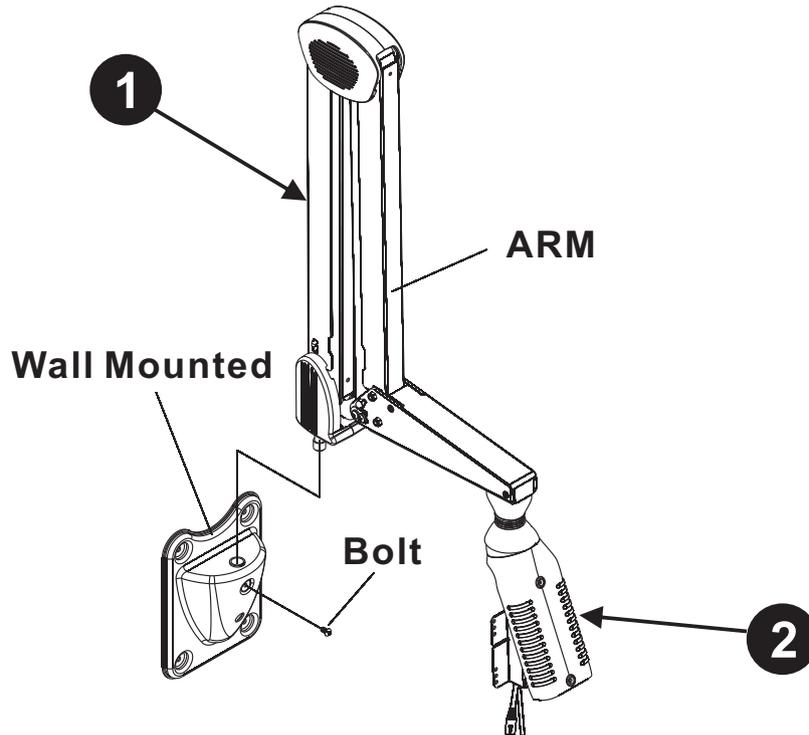
Plug in the main arm in the slot at the wall mounted, Use the fixing Bolts to lock according to the attached picture.
